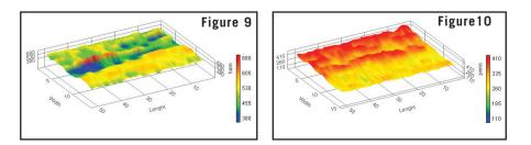
**PC** software allows an overlapping of the moisture and permeability profiles taken by both instruments, allowing an immediate troubleshooting of the felt bands and barring, using the instrument scans taken during the normal routine service, at no extra time
